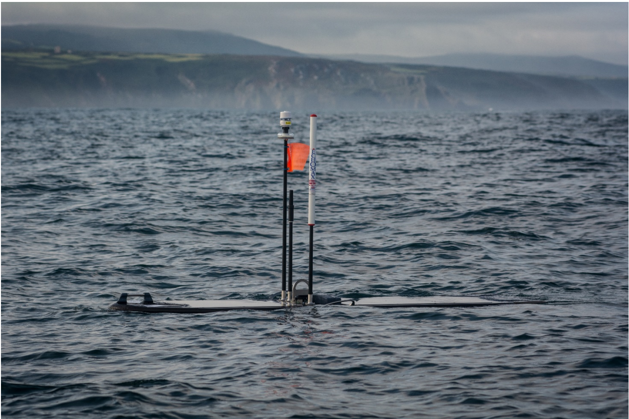
Figure 1: Cefas' Liquid Robotics SV3 Wave Glider deployed for environmental monitoring (Credit: Chris Read (Cefas))
